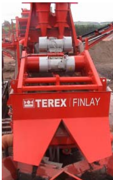
Twin outlet discharge chute
